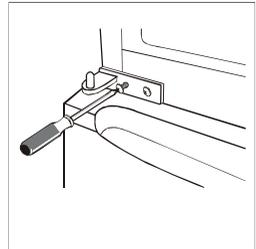
11. Place the upper door back on. Ensure the door is aligned horizontally and vertically so that the seal are closed on all sides before finally tightening the top hinge. Then inert the hinge and screw it to the top of the unit.
