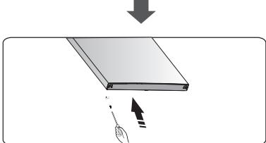
7. Lay the refrigerator on soft foam packaging or similar material. Remove both adjustable bottom feet parts, and the lower hinge part by unscrewing the special flange self-tapping screws.
