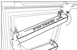
Press the right side of the door shelf inwardly ,while holding the left side . When the notch of the shelf has been detachesd from the refrigerator door , remove the rack obliquely upwardly .
