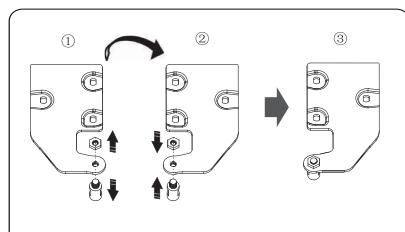
5. Remove the door from the lower hinge
