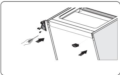
9. Transfer the door to the property position, adjust the lower hinge part, make the hinge axis into the lower hole of the door.
