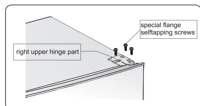
4. Remove the upper hinge axis, transfer it to reversed side and tighten securely, then put it in a safe place.
