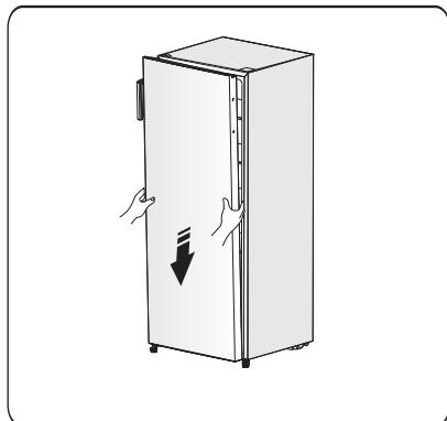
10.Transfer the upper hinge part and make the upper hinge axis into the upper hole of the door, and adjust the position of the door (please support the door with your hand when doing it), fixing the upper hinge part with the special flange self-tapping screws.
