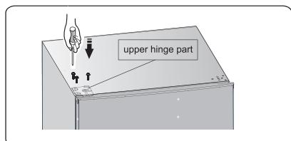
11. Install the screw hole cover on the top right corner of the refrigerator. Install the upper hinge cover (which is in the plastic bag) on the left corner. Put the other upper hinge cover into the plastic bag.
