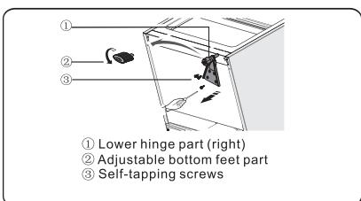
8. Replace the lower hinge part to the left side and fixing it with the special flange self-tapping screws. Replace the adjustable bottom feet parts to another side and fixing it .
